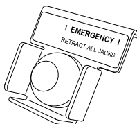
Emergency push button
